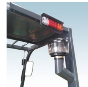
Pre-cleaner engine air intake
