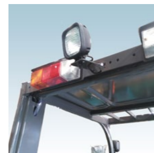
Rear working light
