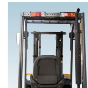
Overhead exhaust system
