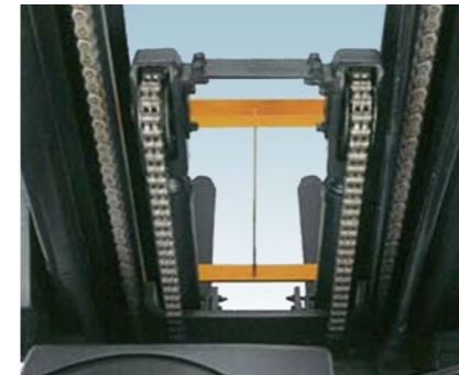
Three-stage mast with four-cylinder mechanism
