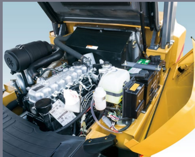
Detachable side covers for convenient inspection and simple maintenance
